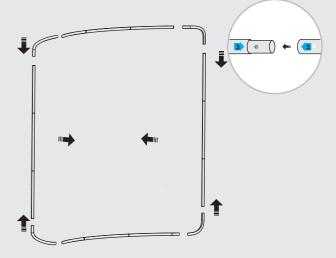
Once you have the frame set, insert the middle pole into the holes in the top & bottom tube.
